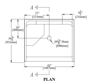
42" [1067mm] Shower w/6" [152mm] Threshold, Molded Soap Ledges, & Molded Seat Located Opposite Valve Wall
